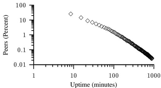
Fig. 4. Uptime distribution for all peers up less than 15 hours using a bin size of 7 minutes, based on data collected between 10/11/2004 1:45pm through 10/12/2004 8:13pm
